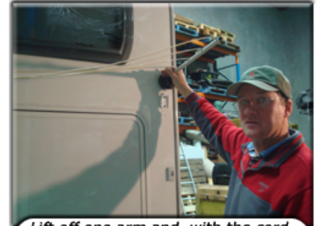
Lift off one arm and, with the cord stretched, rotate arm 180° then walk towards other arm
