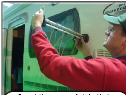
Insert the arm ends into their mating recesses in the arm base section and lock them together
